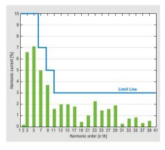
No measures are required for EMC for power levels up to 24 W
